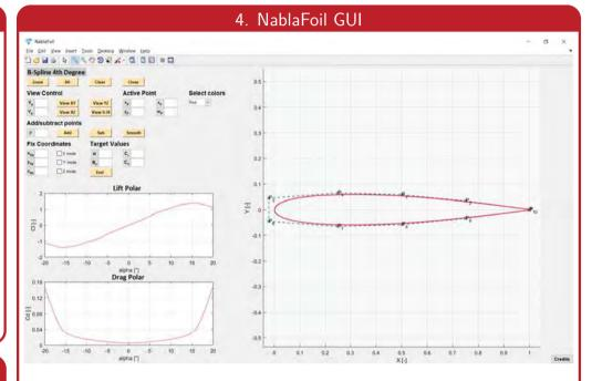
The **NablaFoil** Graphical User Interface shows an interactive draw-mode environment (on the right) linked to two dependent plots of the airfoil polars (on the left). Furthermore, the commands allows to:
